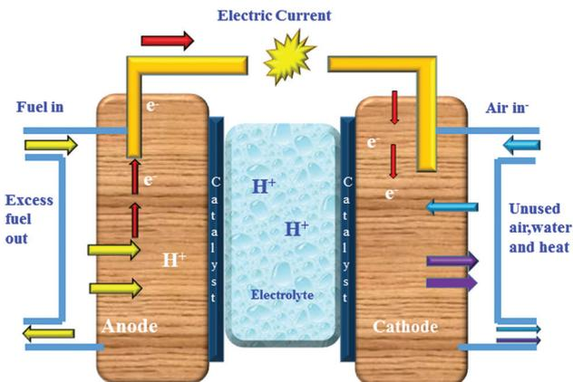
Fig. 1 Schematic illustration of the fuel cell mechanism.
