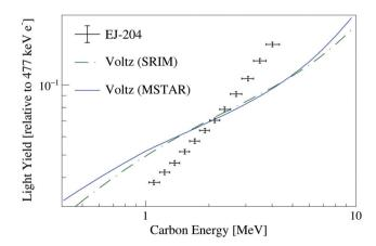
**Fig. 8** EJ-204 carbon light yield data along with Voltz *et al.* models obtained *via* a simultaneous fit of EJ-204 proton and carbon light yield using the SRIM and PSTAR/MSTAR stopping power tables.
