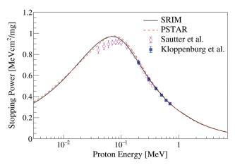
**Fig. 6** Proton stopping power in PVT as calculated by SRIM (black curve) and PSTAR (red dashed curve) libraries. Only two measurements exist in the literature from Kloppenburg *et al.* (filled blue squares) and Sautter *et al.* (open pink circles).
