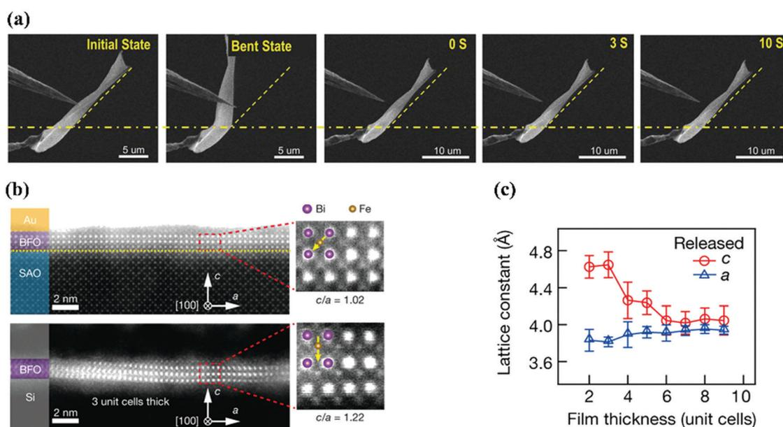
Fig. 4 (a) SEM images of the bending and recovery process at a bending angle of  $40^\circ$  for a BTO nanobelt.<sup>79</sup> (b) Cross-sectional HAADF-STEM images of a BFO thin film (three unit-cell) before (top) and after (bottom) separation from the substrate and (c) the crystal parameters  $a$  and  $c$  as a function of the freestanding BFO film thickness.<sup>80</sup>
