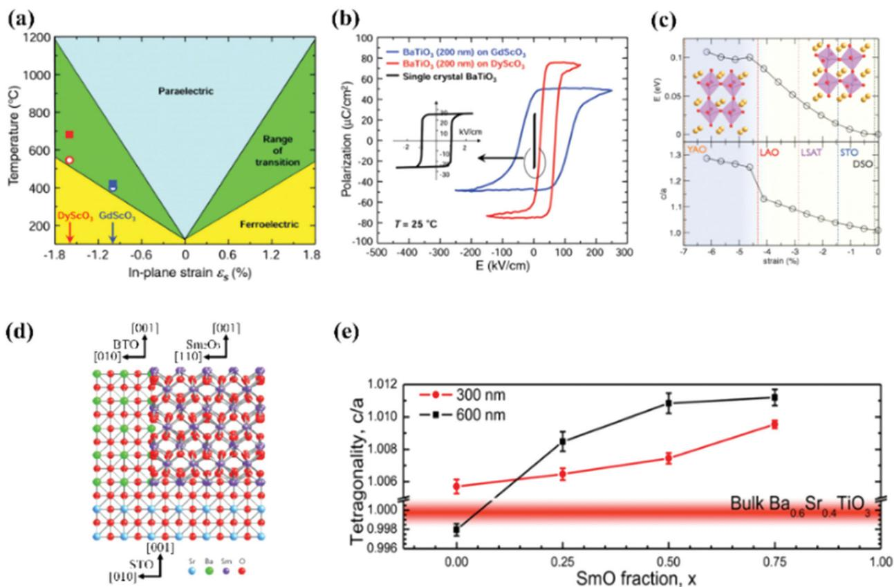
Fig. 2 (a) Misfit strain-temperature phase diagram of BTO and (b)  $P$ - $E$  hysteresis loops of BTO thin films grown on different substrates.<sup>9</sup> (c) Evolution of the energy (top) and  $c/a$  ratio (bottom) as a function of misfit strain for BFO thin films.<sup>7</sup> (d) Schematic crystallographic model of vertical strain between Sm<sub>2</sub>O<sub>3</sub> and BTO.<sup>65</sup> (e) Tetragonality ( $c/a$ ) in BSTO thin films versus Sm<sub>2</sub>O<sub>3</sub> content.<sup>66</sup>
