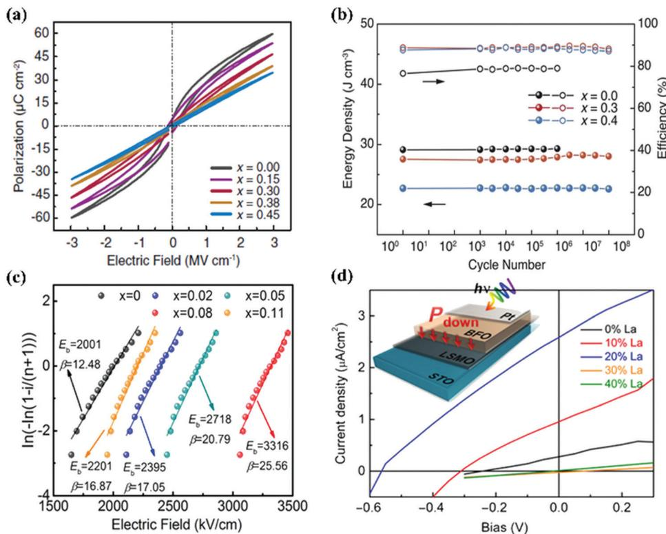
Fig. 1 (a) The  $P$ - $E$  curves of Sm-doped BFO-BTO thin films with various Sm content.<sup>25</sup> (b) A cyclic fatigue test for energy storage density and efficiency of  $(0.55-x)\text{BFO}-x\text{BTO}-0.45\text{STO}$  solid-solution thin films with various  $x$  values.<sup>26</sup> (c) The breakdown strengths of BLT- $x\text{BFO}$  thin films were analyzed by two-parameter Weibull distribution.<sup>27</sup> (d) Photocurrent density-voltage curves of La-substituted BFO films.<sup>28</sup>
