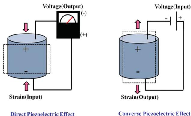
Fig. 7 Schematic diagram of the positive piezoelectric effect and the inverse piezoelectric effect.<sup>130</sup>
