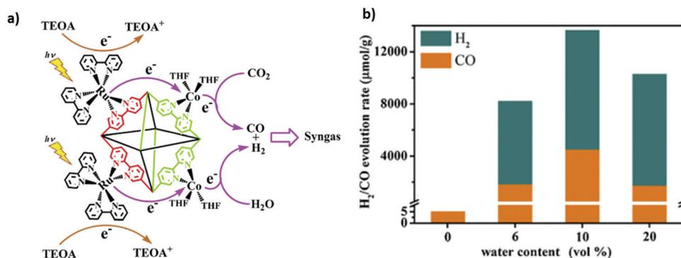
Fig. 8 (a) Proposed mechanism for photocatalytic syngas production with  $(\text{Co/Ru})_n\text{-UiO-67(bpydc)}$  as the catalyst under the visible light irradiation. (b) Time profile of  $\text{H}_2$  and  $\text{CO}$  evolution rate. Reproduced and modified with permission.<sup>39</sup> Copyright 2019, Elsevier.
