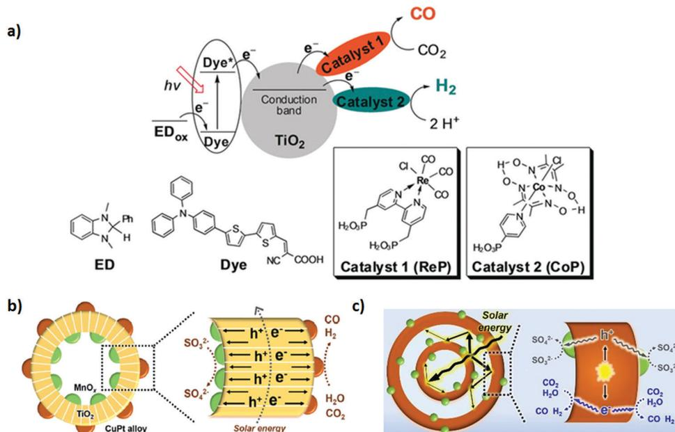
**Fig. 3** (a) Schematic representation of the heterogeneous ternary photocatalytic system for syngas production. Reproduced and modified with permission.<sup>115</sup> Copyright 2017, Wiley-VCH. (b) Mechanism of the photocatalytic CRR driven by MTCP-MSs. Reproduced and modified with permission.<sup>117</sup> Copyright 2018, Royal Society of Chemistry. (c) The photoreaction processes of D-CMH. Reproduced and modified with permission.<sup>114</sup> Copyright 2020, Royal Society of Chemistry.
