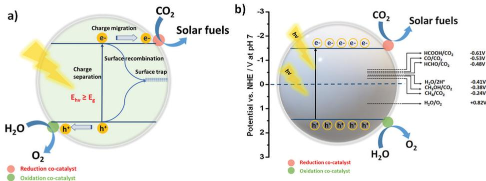
Fig. 1 (a) Schematic illustration of the elementary processes of photogenerated charges over the photocatalytic surface. (b) Schematic illustration of photocatalytic  $\text{CO}_2$  and  $\text{H}_2\text{O}$  conversion over a semiconducting photocatalyst for solar fuel production mediated by suitable redox co-catalysts.
