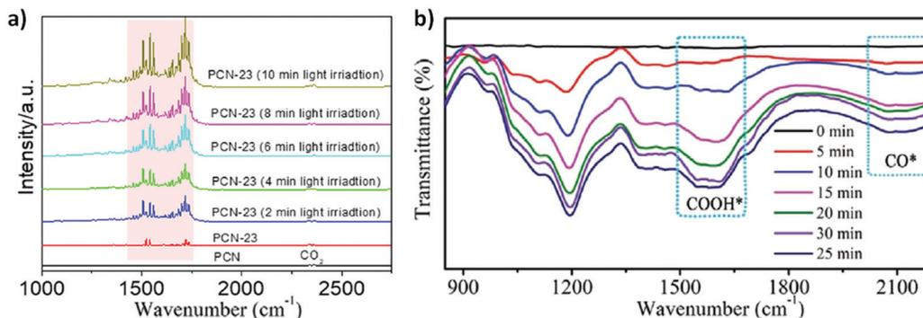
Fig. 11 *In situ* DRIFTS spectra illustrating the photocatalyzed CO<sub>2</sub> adsorption–activation over the surface of (a) PCN and defect rich PCN-23 (reproduced and modified with permission.<sup>42</sup> Copyright 2021, Elsevier) and (b) 3DOM CdSQD/NC (reproduced and modified with permission.<sup>20</sup> Copyright 2021, Wiley-VCH).
