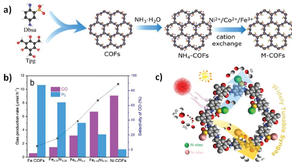
**Fig. 10** (a) Synthesis of M-COFs with 2,4,6-triformylphloroglucinol (Tpg) and 2,5-diaminobenzenesulfonic acid (Dbsa) as the precursors. (b) The dependence of CO/H<sub>2</sub> ratios of metals in a series of Fe/Ni-COF samples in low-concentration CO<sub>2</sub>. (c) Schematic scheme for CO<sub>2</sub> reduction into CO and H<sub>2</sub>. Reproduced and modified with permission.<sup>41</sup> Copyright 2020, Wiley-VCH.
