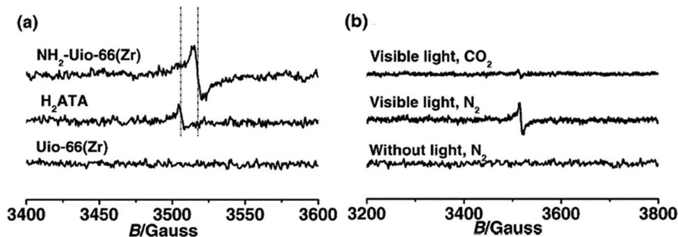
Fig. 12 (a) EPR spectra of NH<sub>2</sub>-Uio-66(Zr), Uio-66(Zr), and H<sub>2</sub>ATA under visible light irradiation. (b) EPR spectra of NH<sub>2</sub>-Uio-66(Zr) in different atmospheres under visible light irradiation. Reproduced and modified with permission.<sup>204</sup> Copyright 2013, Wiley-VCH.
