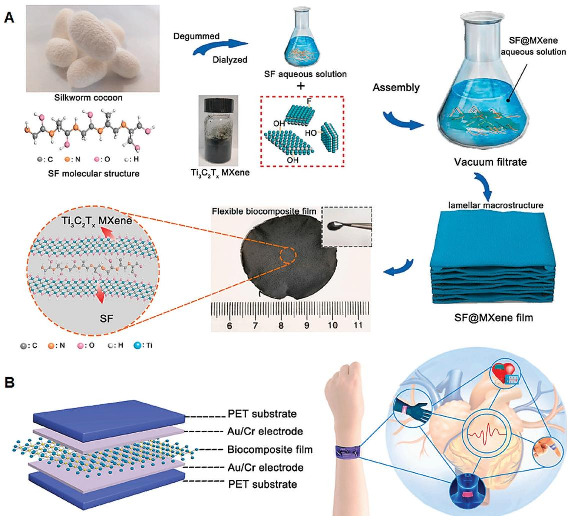
**Fig. 2** (A) The preparative process of flexible silk fibroin (SF)@ $\text{Ti}_3\text{C}_2\text{T}_x$  MXenes with high biocompatibility, and (B) the design of MXene film-based flexible pressure sensor with high sensitivity and suitable mechanical properties for human health detection applications. Reproduced with permission from ref. 66 Copyright 2020 Elsevier.
