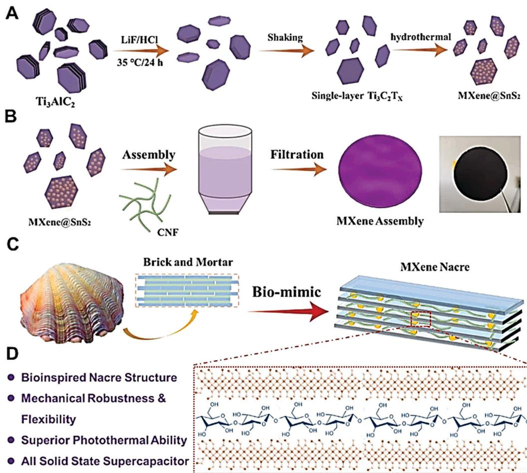
Fig. 3 Preparative process for bioinspired MXene-based structures constructed from  $\text{Ti}_3\text{C}_2\text{T}_x$  nanosheets and  $\text{SnS}_2$  nanoparticles. Reproduced with permission from ref. 68 Copyright 2021 Elsevier.
