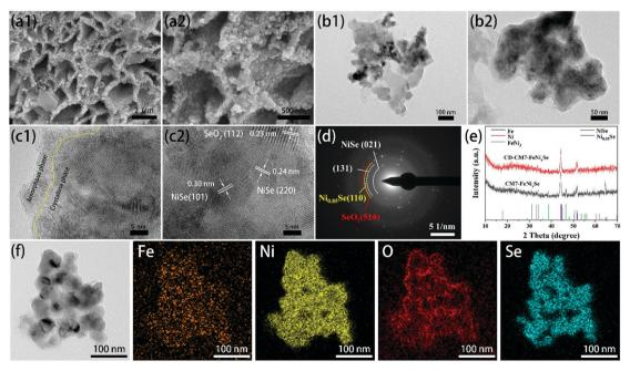
Fig. 4 (a1 and a2) SEM images, (b1 and b2) TEM images, (c1 and c2) HRTEM images, (d) SAED patterns, (e) XRD pattern and (f) EDX elemental mapping of CM7-FeNi<sub>x</sub>Se after the chronopotentiometry test (CD-CM7-FeNi<sub>x</sub>Se) at constant current densities of 20 mA cm<sup>-2</sup> for 10 h.
