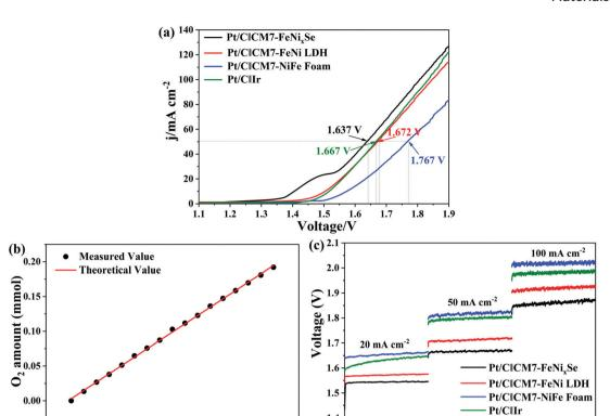
Fig. 6 (a) Polarization curves for overall water splitting. (b) Amounts of gas experimentally measured and theoretically calculated vs. time for the electrolyzer Pt/C||CM7-FeNi, Se at 10 mA cm<sup>-2</sup>. (c) Chronopotentiometry curves tested at constant current densities of 10, 50 and 100 mA cm<sup>-2</sup>
