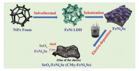
Scheme 1 Schematic illustration of the formation process of hierarchical SeO<sub>x</sub>/FeNi<sub>x</sub>Se (CMy-FeNi<sub>x</sub>Se).
