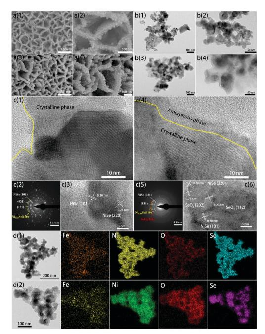
Fig. 1 (a1 and a2) SEM images, (b1 and b2) TEM images, (c1 and c3) HRTEM images, (c2) SAED pattern and (d1) EDX elemental mapping of FeNixSe; (a3 and a4) SEM images, (b3 and b4) TEM images, (c4 and c6) HRTEM images, (c5) SAED pattern and (d2) EDX elemental mapping of CM7-FeNi<sub>x</sub>Se.
