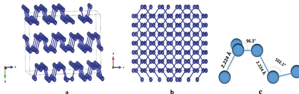
Fig. 1 (a) The crystal structure of BP; (b) crystal structure view along the *b*-axis; (c) bond length and bond angles of phosphorene.<sup>47</sup>
