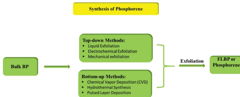
Fig. 2 Different preparative methods of FLBP or phosphorene.<sup>94</sup>
