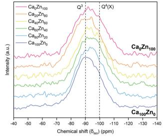
Fig. 8  $^{29}$ Si MAS NMR spectra for the  $Ca_xZn_y$  glass series overlaid with chemical shifts approximately representative of  $Q^3$  and  $Q^4(X)$  (where X is a network former other than Si) species. Indicative location of  $Q^3$  and  $Q^4(X)$  species are shown.
