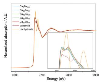
Fig. 1 XANES spectra for the  $Ca_xZn_y$  glass series, compared with the Zn standards willemite (Zn<sub>2</sub>SiO<sub>4</sub>) and hardystonite (Ca<sub>2</sub>ZnSi<sub>2</sub>O<sub>7</sub>).
