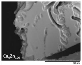
Fig. 10 Scanning Electron Microscopy images of Ca<sub>100</sub>Zn<sub>0</sub> and Ca<sub>0</sub>Zn<sub>100</sub> obtained after dissolution under dynamic conditions.
