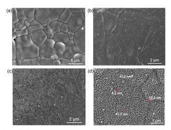
Fig. 4 (a) SEM image of the bare NF, (b) anodized NF substrate for 2 h, (c) HS-Te-NiCo-LDH/NiO/NF, and (d) enlarged SEM image of HS-Te-NiCo-LDH/NiO/NF.
