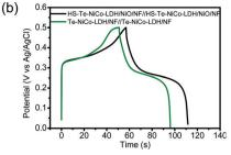
Fig. 6 Electrochemical measurements of the HS-Te-NiCo-LDH/NiO/NF, Te-NiOH/NiO/NF, HS-NiCo-LDH/NiO/NF, Te-CoOH/NiO/NF, Te-CoOH/NiO/NF, Te-NiCo-LDH/NiO/NF, Te-NiCo-LDH/ electrodes in 2 mol L<sup>-1</sup> KOH aqueous solution. (a) CV curves at 5 mV s<sup>-1</sup>, (b) GCD curves of HS-Te-NiCo-LDH/NiO/NF//HS-Te-NiCo-LDH/NiO/NF, and Te-NiCo-LDH/NF//Te-NiCo-LDH/NF at 10 A g<sup>-1</sup>.
