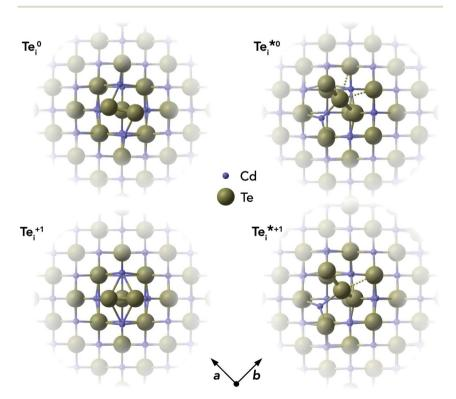
Fig. 3 Atomic structures of ground-state ( $Te_i^{0/+1}$ ) and metastable ( $Te_i^{*0/+1}$ ) tellurium interstitials in CdTe, looking down the [001] axis. Atoms sized according to their formal ionic radii.<sup>31</sup> Te anions are shown in gold and Cd cations in purple.
