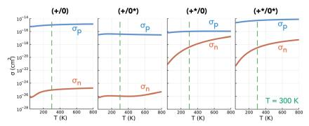
Fig. 6 Electron and hole capture cross-section ( $\sigma_{\rm n}$  and  $\sigma_{\rm p}$ ) as functions of temperature T for the Te<sub>i</sub> (+(\*)/0(\*)) charge transition levels in CdTe. Room temperature ( $T=300~{\rm K}$ ) denoted by the dashed green line as a guide for typical solar cell operating conditions.
