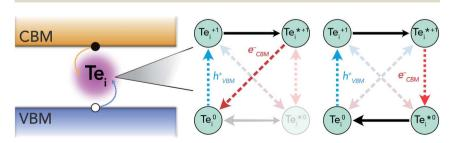
Fig. 7 Schematic of the proposed non-radiative recombination mechanism at tellurium interstitials in CdTe. Red/blue arrows denote electron/hole capture, and black arrows indicate internal conversion reactions.
