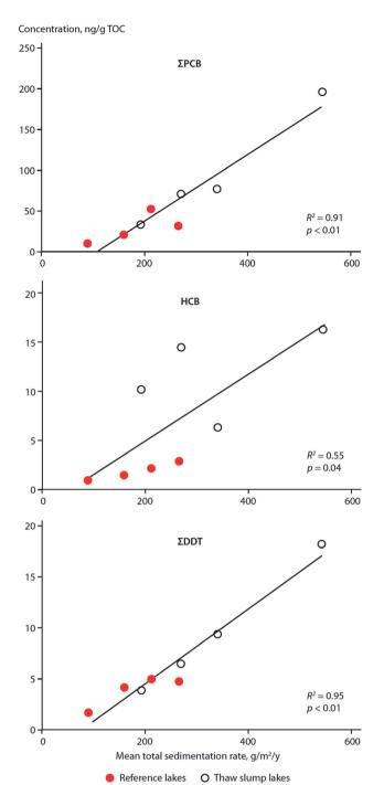
Fig. 15 Concentrations (ng g $^{-1}$  TOC) of  $\Sigma$ PCBs, HCB and  $\Sigma$ DDT in sediments from eight study lakes, including reference lakes (red points) and lakes affected by thaw slumps (white points) in tundra uplands adjacent to the Mackenzie Delta, Canada, plotted *versus* the mean total sedimentation rate (g per m $^2$  per year) in each lake. Redrawn from Eickmeyer *et al.* (2016). $^{185}$
