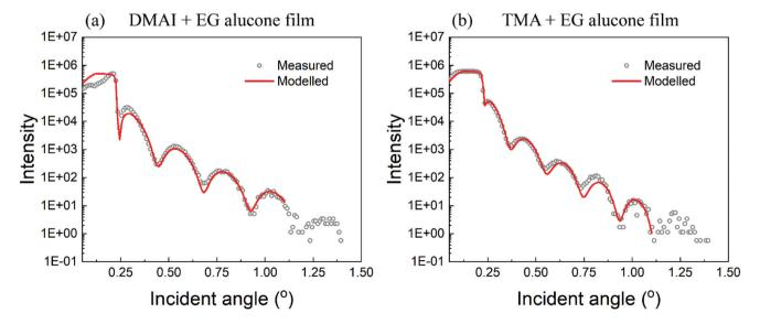
Fig. 5 XRR scans of the alucone films prepared using (a) DMAI and (b) TMA. The fitted intensity is shown in red. The extracted density of the DMAI + EG film  $\approx$  1.72 g cm<sup>-3</sup> and that of TMA + EG film  $\approx$  1.75 g cm<sup>-3</sup>.
