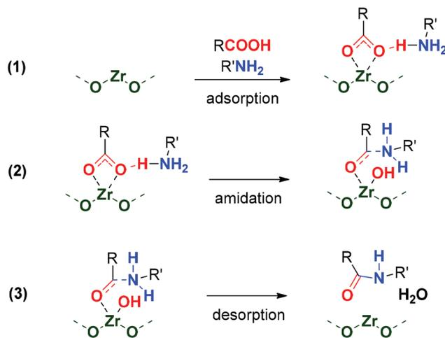
**Scheme 2** Proposed mechanism of amide bond formation with Zr-MOFs.
