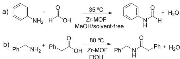
**Scheme 1** (a) Formylation of aniline, and (b) reaction between phenylamine and phenylacetic acid catalysed by the CUSs of the Zr-MOFs MOF-808 and UiO-66.<sup>27,28</sup>
