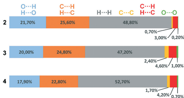
Fig. 3 Representation of the composition of the Hirshfeld surface from different intermolecular contacts.
