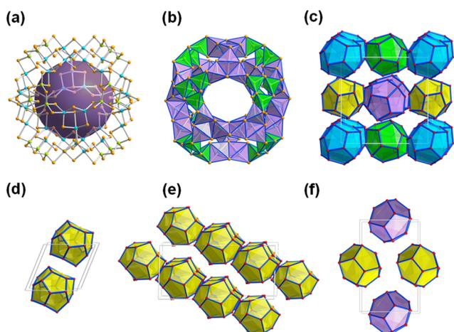
Fig. 2 Molecular structure of the superspherical 'zeoball' cluster anion [Sn<sub>36</sub>Ge<sub>24</sub>Se<sub>132</sub>]<sup>24-</sup>, with the purple sphere representing the cavity inside the anion (a), polyhedral representation of the 'zeoball' anion (b), crystal packing pattern of the anions with overall pentagonal dodecahedral topology in the prototypical salt (c) and in three further 'zeoball' salts (d-f). Counterions are omitted for clarity. Color code: Ge-lime, Sn-turquoise, Se-orange.
