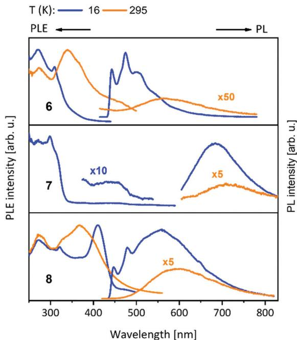
Fig. 6 Solid state excitation and emission spectra of bis-NHC<sup>bipy</sup> ( $L^2$ ) metal complexes **6–8**. PL was excited at  $\lambda_{exc} = 300$  nm for **6, 8** and  $\lambda_{exc} = 320$  nm for **7**. PLE spectra were recorded at  $\lambda_{em} = 500/560$  nm (**6**),  $\lambda_{em} = 700/750$  nm (**7**) and  $\lambda_{em} = 550/600$  nm (**8**) at low/elevated temperatures respectively.<sup>42</sup>
