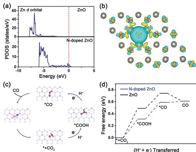
Fig. 4 DFT calculations. (a) Calculated PDOS of Zn *d*-orbital in N-doped and undoped ZnO nanorods, (b) differential charge diagram of ZnO with nitrogen dopant, the gray, red, and white spheres represent Zn, O, and N atoms, respectively. (c) A possible reaction path for CO<sub>2</sub>RR to CO on N-doped ZnO nanorods, and (d) DFT free energy profiles of CO<sub>2</sub>RR to CO.
