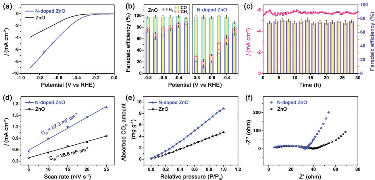
Fig. 3 The CO<sub>2</sub>RR performance of ZnO and N-doped ZnO nanorods. (a) LSV curves, (b) FEs of CO, CH<sub>4</sub> and H<sub>2</sub> at various applied potentials, (c) stability test for N-doped ZnO nanorods at  $-0.7$  V vs. RHE and the FE variation for CO production, (d) charging current density differences  $j$  plotted against the scan rates, (e) CO<sub>2</sub> adsorption isotherms, and (f) Nyquist plots of EIS.
