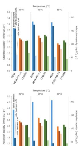
Fig. 20 Effect of propylene oxide modification of TEPA- and PEHA-based adsorbents on  $CO_2$  adsorption under 95%  $CO_2$  in 25, 55, and 85 °C for 3 h before and after treatment under air or  $N_2$  at 100  $^{\circ}\text{C}$  for 20 h. Comparison with LPEI25k/50S. Reproduced with permission from ref. 70. Copyright 2019, John Wiley and Sons.
