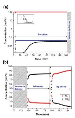
Fig. 25 (a) Breakthrough profile of PEI-functionalised cellulose acetate/silica fibres during  $CO_2$  adsorption under dry 380 ppm  $CO_2/395$  ppm He/balance  $N_2$  at 35 °C. (b) Concentration profiles during the 'self-sweep' and  $N_2$  sweep stages of desorption. Reprinted with permission from ref. 39. Copyright (2019) American Chemical Society.
