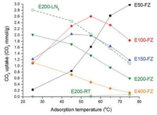
Fig. 11 Variation in  $CO_2$  capacity with temperature for different amine/cross-linker compositions. Adsorption under  $10\% CO_2$  for 3 hours. Reproduced from ref. 117 with permission from the Royal Society of Chemistry.
