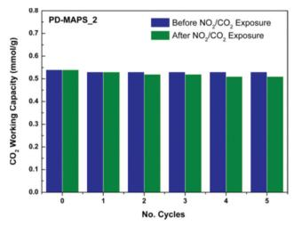
Fig. 23 CO<sub>2</sub> working capacity of the secondary amine-grafted adsorbent before and after exposure to 20 ppm of NO<sub>2</sub> in 10% CO<sub>2</sub>/N<sub>2</sub> at 35 °C. Reprinted with permission from ref. 151. Copyright (2014) American Chemical Society.
