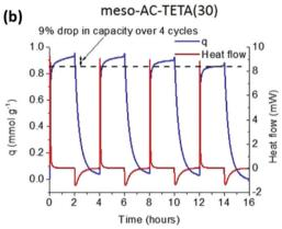
Fig. 18 Cyclic CO<sub>2</sub> adsorption-desorption experiments at 75 °C on (a) meso-AC-PEI600(100), and (b) meso-AC-TETA(30). Reprinted from ref. 130, Copyright (2015), with permission from Elsevier.
