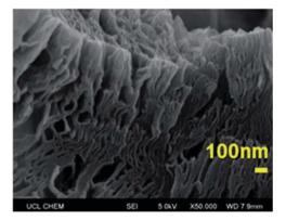
**Fig. 5** SEM micrograph of exfGO-D\_7.0TETA, exfoliated graphene-oxide impregnated with 7.0 g  $\rm g^{-1}$  TETA. Reproduced from ref. 94 with permission from the Royal Society of Chemistry.
