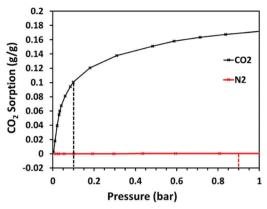
**Fig. 16** Selectivity of  $CO_2$  uptake of BC40. Single-component  $CO_2$  and  $N_2$  sorption (g g<sup>-1</sup>) at 90 °C in the low-pressure range. The dashed lines indicate the corresponding interpolated uptakes at the representative pressures of flue gas: 0.10 bar  $CO_2$  and 0.90 bar  $N_2$ . Reprinted with permission from ref. 116. Copyright (2019) American Chemical Society.
