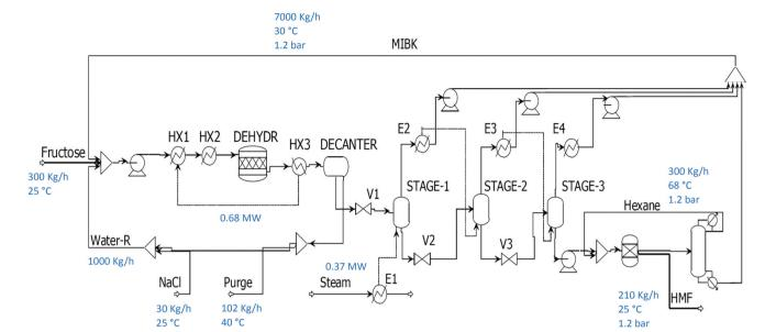
Fig. 3 Process flowsheet for the synthesis and isolation of HMF using a water-MIBK system.
