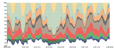
Fig. 1 Energy mix of the German power grid throughout August 2020 in fractions of the total demand. The maximum power demand was 74 GW. The negative values represent the export, the purple elements the net import of power. Colour coding: yellow solar, light green wind, light blue pumped hydro, orange gas, dark brown coal, light brown lignite, red nuclear, green biomass, dark blue hydro. (Source: Fraunhofer ISE, Energy Charts.)
