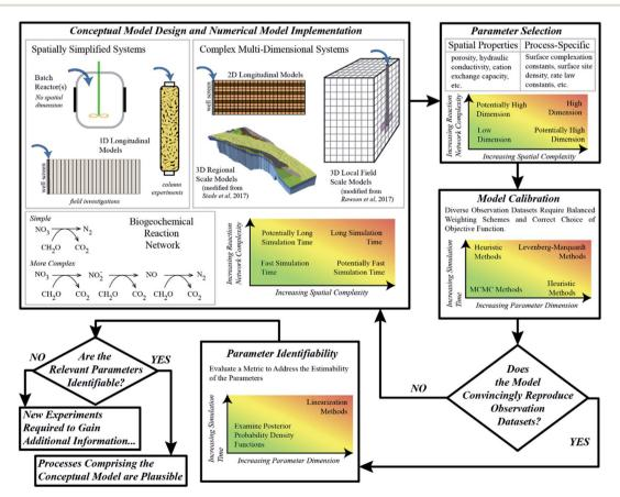
Fig. 1 Flow chart of iterative model development procedure.
