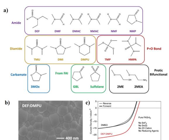
Fig. 4 (a) 16 nonsulfoxide solvents that formed stable perovskite solution divided into groups according to the functional group. (b) SEM images of the DEF:DMPU film. (c) J-V curves of FASnl<sub>3</sub> without any additives in DEF:DMPU against DMSO.<sup>78</sup> Reproduced with permission Copyright 2021, American Chemical Society
