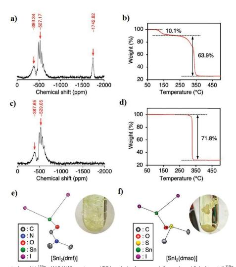
Fig. 2 Purified  $Snl_2$  reagents, (a and b)  $^{119}Sn$  MAS NMR spectra, and TGA analysis of commercially purchased  $Snl_2$ . (c and d)  $^{119}Sn$  MAS NMR spectra and TGA analysis of purified  $Snl_2$  using the vacuum sublimation method. (e and f) Structural illustrations of  $[Snl_2(DMF)]$  and  $[Snl_2(DMSO)]$ . Reproduced with permission Copyright 2020, American Chemical Society.
