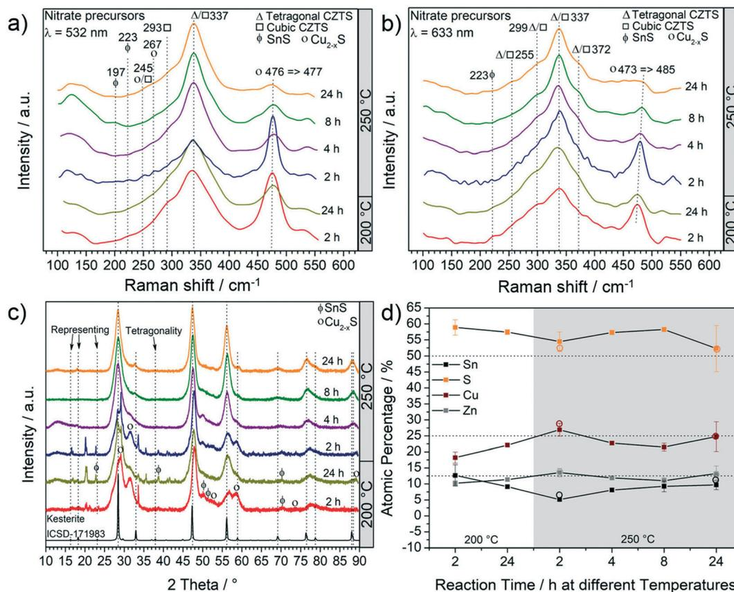
**Fig. 1** Characterization of particles obtained at different temperatures and for different time lengths. Raman analysis using (a) green and (b) red lasers; (c) XRD patterns and (d) EDX analysis: solid square data points represent SEM-EDX analysis and the empty circle data points represent TEM-EDX analysis. The products mainly consist of CZTS phase with  $\text{Cu}_{2-x}\text{S}$  and SnS as the other main by-products.
