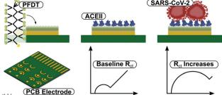
Scheme 1 Top - Two stage functionalisation process of the PFDT-ACE sensor and virus binding. Bottom - The electrode chip and the resulting R<sub>CT</sub> increase upon virus recognition.
