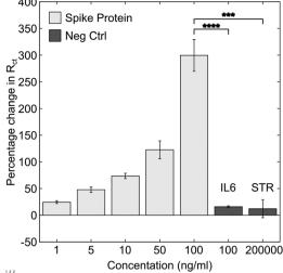
Fig. 1 Dose response curve for PFDT-ACE2 modified sensors when incubated for 30 min with solutions of recombinant SARS-CoV-2 spike protein. Negative controls: 100 ng mL<sup>-1</sup> IL-6 and 200 μg mL<sup>-1</sup> streptavidin. N = 8 & Error Bars = SE.
