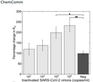
**Fig. 2** Dose response following incubation of PFDT-ACE2 modified sensor with inactivated SARS-CoV-2 molecular standards kit. Viral concentration is expressed in copies  $\mathrm{mL}^{-1}$  which is the result of sample quantification following viral inactivation using digital PCR. N=6~& Error Bars = SE.
