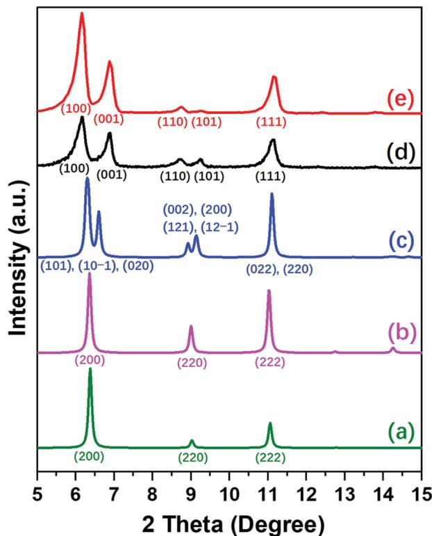
Fig. 2 PXRD patterns of simulated (a) as-made ITQ-21, (b) dehydrated PKU-14, (c) as-made PKU-14, and experimental (d) as-made NUD-3 and (e) calcined NUD-3. Each peak ranging from  $2\theta$  5–15° is marked with its Miller index.
