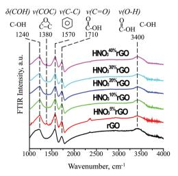
Fig. 4 FTIR spectra of the initial and HNO3-treated rGO materials.
