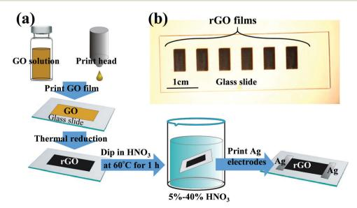
Fig. 1 (a) Illustration of experimental procedures to fabricate inkjet-printed and HNO3-treated rGO films and (b) optical image of rGO films.
