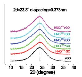
Fig. 6 XRD patterns of the initial and HNO<sub>3</sub>-treated rGO materials.
