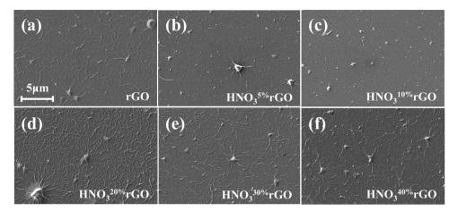
Fig. 2 SEM images of (a) rGO and (b-f) HNO<sub>3</sub>-treated rGO films on Si wafers
