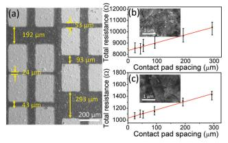
Fig. 4 SEM image of Au/Ti contact pads on r-Ti<sub>3</sub>C<sub>2</sub>T<sub>x</sub> films on SiO<sub>2</sub>/Si (a), plots of total resistance vs. contact pad spacing of (b) Ti<sub>3</sub>C<sub>2</sub>T<sub>x</sub> and (c)  $r-Ti_3C_2T_x$  films on  $SiO_2/Si$ . Insets in figures b and c are the high magnification SEM images of the corresponding films.
