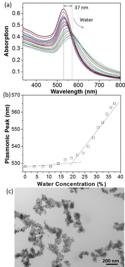
Fig. 2 (a) UV-vis spectra of PS<sub>65</sub>-NHC modified AuNPs in THF when titrating with water. The spectra were collected by adding 80  $\mu$ L of water each time into 2 mL of the THF solution of AuNPs. (b) Plotting the plasmonic peak of PS<sub>65</sub>-NHC modified AuNPs as a function of water concentration to determine the critical water concentration. (c) TEM image of PS<sub>65</sub>-NHC modified AuNPs in THF/water (1:1 vol) mixture.
