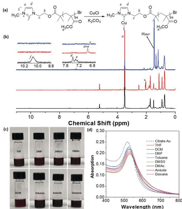
Fig. 4 (a) Synthesis of PMMA<sub>85</sub>-NHC-Cu(I) using an imidazole-containing ATRP initiator. (b) <sup>1</sup>H NMR spectra of PMMA<sub>85</sub>-Im (black, bottom), PMMA<sub>85</sub>-NHC-Cu(I) (red, middle) and PMMA<sub>85</sub>-NHC-Au (blue, top) in CD<sub>2</sub>Cl<sub>2</sub>. (c) Images showing PMMA<sub>85</sub>-NHC-Au dispersed in various organic solvents. (d) UV-vis spectra showing the SPR absorption of PMMA<sub>85</sub>-NHC-Au in various solvents.
