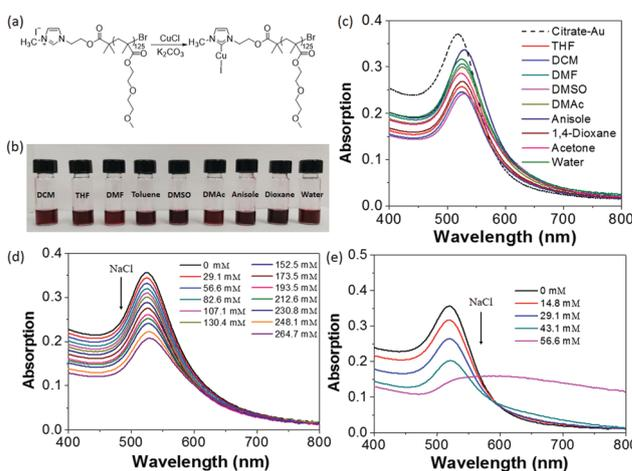
Fig. 5 (a) Synthesis of P(MEO<sub>2</sub>MA)<sub>125</sub>-NHC-Cu(I) using an imidazole-containing ATRP initiator. (b) Image showing solutions of P(MEO<sub>2</sub>MA)<sub>125</sub>-NHC-Au in various organic solvents and water. (c) UV-vis spectra showing the SPR peaks of AuNPs dispersed in various solvents. (d and e) Titration experiments showing the stability of P(MEO<sub>2</sub>MA)<sub>125</sub>-NHC-Au (d) and citrate-capped AuNPs (e) upon addition of 1 M NaCl.
