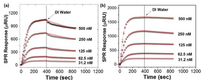
Fig. 6 SPR traces showing the binding kinetics of (a) PMEO<sub>2</sub>MA<sub>125</sub>-NHC-Cu(I) and (b) PMEO<sub>2</sub>MA<sub>174</sub>-SH to Au. After the flow of polymer solution, the DI water was flowed over the Au sensor to trace the dissociation. The thin red lines are the fit curves of the kinetic data.
