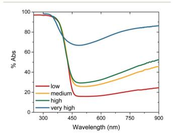
Fig. 1 UV-visible absorption spectra, determined from integrating sphere measurements of transmission and reflectance, for WO<sub>3</sub> films without annealing ('very high' [V<sub>O</sub>], blue), after acid treatment ('high'  $[V_O]$ , green), after 2 hour annealing ('medium'  $[V_O]$ , yellow) and after 12 hour annealing ('low'  $[V_{\Omega}]$ , red).
