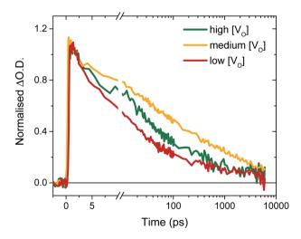
Fig. 5 Normalised ultrafast transient absorption kinetics in 0.1 M H<sub>2</sub>SO<sub>4</sub>, probing the electron decay at 700 nm from ~200 femtoseconds to 6 ns after excitation with 355 nm (0.2 mJ cm<sup>-2</sup>, no bias) for 'high' to 'medium' and 'low' [Vo] doping concentrations.
