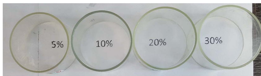
Fig. 30 Photographs of films containing 5, 10, 20, and 30% curing agent, respectively. 141
