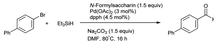
Scheme 67 Synthesis of aldehydes from aryl halides.
