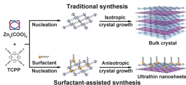
Fig. 12 Preparation of MOFs by traditional synthesis and surfactant-assisted synthesis. In the traditional method, isotropic growth produces large crystals of MOFs, while in the surfactant-assisted synthesis, the surfactant causes anisotropic growth of MOFs to form uniform ultra-thin MOF nanosheets. 139 Blue and purple are used to draw MOF layers separately. Copyright, 2015 Wiley-VCH.
