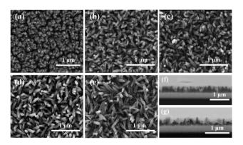
Fig. 2 SEM images of (a) pristine hematite, (b) H/UCDs (5), (c) H/UCDs (10), (d) H/UCDs (15), (e) H/UCDs (20); cross-section SEM images of the (f) pristine hematite and (g) H/UCDs (10) photoanodes.
