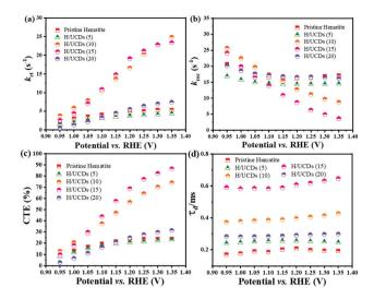
Fig. 7 (a)  $k_{\rm tr}$ , (b)  $k_{\rm rec}$ , (c) charge transfer efficiency (CTE), and (d) diffusion lifetime of the photogenerated charge carriers calculated from IMPS plots.
