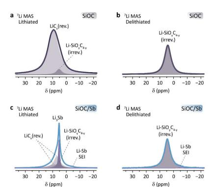
Fig. 6 <sup>7</sup>Li MAS NMR (12 kHz) spectra of (a and c) lithiated and (b and d) delithiated SiOC and SiOC/Sb, respectively.
