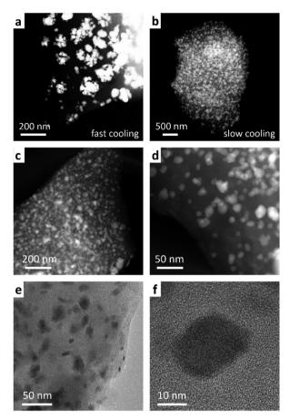
Fig. 3 HAADF STEM images of a SiOC/Sb obtained using a cooling rate of (a) 5 °C min<sup>-1</sup> and (b-d) 1 °C min<sup>-1</sup>, respectively. EDXS analysis of SiOC/Sb indicates that the bright spots on HAADF-STEM images represent Sb NPs (Fig. S1 and S2†) (e and f) TEM images of SiOC/Sb.
