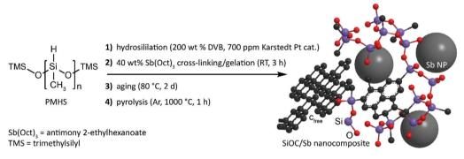
Fig. 1 Schematics of the synthetic protocol of SiOC/Sb nanocomposite.
