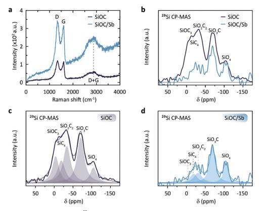
Fig. 4 (a) Raman spectra of SiOC and SiOC/Sb. (b) <sup>29</sup>Si CP-MAS NMR spectra of SiOC and SiOC/Sb. The intensities are scaled to the SiO<sub>4</sub> peak intensity. (c) Fitted <sup>29</sup>Si CP-MAS NMR spectrum of SiOC. (d) Fitted <sup>29</sup>Si CP-MAS NMR spectrum of SiOC/Sb.
