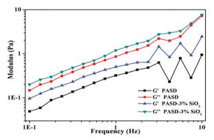
Fig. 13 Storage moduli and loss moduli as a function of frequency for PASD and PASD-3%SiO<sub>2</sub>.
