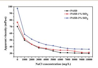
Fig. 10 Effect of the NaCl concentratione on apparent viscosity of PASD and PASD-SiO<sub>2</sub>
