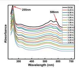
Fig. 2 The UV absorption spectra of DWPU prepolymers reacted at 70 °C.
