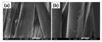
Fig. 10 SEM micrographs of polyester fabrics (a) and fabrics coated with D<sub>2</sub>WPU (b). The scale bars are 10 μm.
