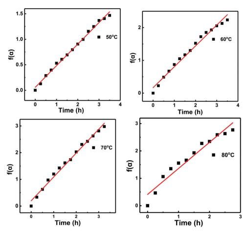
$f(\alpha)$  vs. time linear fitting curves at different temperatures
