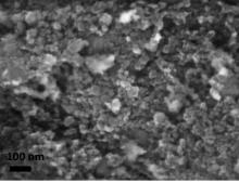
Fig. 1 Scanning electron micrographs of (left) CeO<sub>2</sub>(aero) and (right) CeO<sub>2</sub>(partic).
