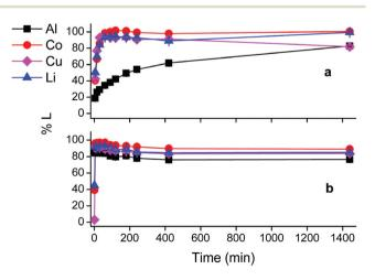
Fig. 6 Comparison between leaching with leaching of  $LiCoO_2$  by DES and HCl solution. Top: DES leaching (ChCl:CA 2:1 +35 wt% H<sub>2</sub>O). Bottom: Leaching with HCl 1 mol L<sup>-1</sup>. Leaching parameters: S:L = 20 g L<sup>-1</sup>, 40 °C, Al:LiCoO<sub>2</sub> = 12 wt%, Cu:LiCoO<sub>2</sub> = 24 wt% at a stirring rate of 900 rpm.
