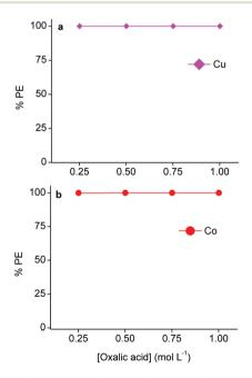
**Fig. 9** Efficiencies of stripping precipitation of metal oxalates at different oxalic acid concentrations. (a) Cu(I/II) oxalate formation by stripping from loaded 60 vol% LIX 984 in an aliphatic diluent and (b) cobalt(II) oxalate formation by stripping from loaded undiluted water-presaturated A336. The loaded LIX 894 and A336 contained 4.7 g  $L^{-1}$  Cu(I/II) and 9.8 g  $L^{-1}$  Co(III). Phase ratio = 1:1, equilibration = 30 min, shaking speed = 2250 rpm, room temperature.
