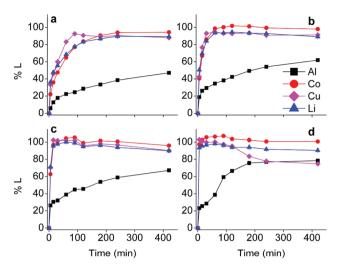
Fig. 1 Leaching efficiencies (%L) of LiCoO $_2$  + Al + Cu mixtures in choline chloride–citric acid DES as a function of time at different temperatures. Temperatures: room temperature (left above, a), 40 °C (right above, b), 60 °C (left below, c) and 80 °C (right below, d). DES: ChCl : CA 2:1+35 wt%  $H_2O$ . Leaching parameters: S:L=20 g  $L^{-1}$ , Al : LiCoO $_2=12$  wt%, Cu : LiCoO $_2=24$  wt% at 900 rpm.
