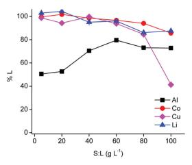
Fig. 2 Variation of the solid-to-liquid ratio (S:L) during leaching by choline chloride-citric acid DES. Composition of the DES: ChCl: CA 2:1 +35 wt% H<sub>2</sub>O. Leaching parameters: 1 h at 40 °C, Al: LiCoO<sub>2</sub> = 12 wt%, Cu :  $LiCoO_2 = 24$  wt% at 900 rpm.
