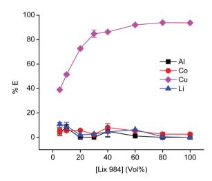
Fig. 8 Optimisation of the LIX 984 concentration in the aliphatic diluent during extraction of metals from the PLS. Initial metal concentrations in the PLS: Al( $\parallel$ ) 1.0 g L<sup>-1</sup>, Co( $\parallel$ ) 12.1 g L<sup>-1</sup>, Cu( $\parallel$ / $\parallel$ ) 4.7 g L<sup>-1</sup> and Li ( $\parallel$ ) 1.1 g L<sup>-1</sup>. Equal phase ratio was used. Equilibration time = 30 min, shaking speed = 2250 rpm, room temperature.
