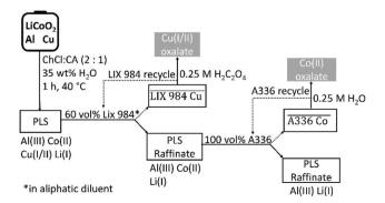
Fig. 10 Conceptual flow sheet for the solvometallurgical recovery of cobalt(II) from LiCoO<sub>2</sub> by a choline chloride-citric acid DES.
