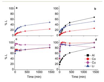
Fig. 3 Comparison of the effects of current collector metals on the leaching of lithium cobalt oxide by choline chloride-citric acid DES. Conditions: Only LiCoO<sub>2</sub> (left above, a), LiCoO<sub>2</sub> with Al (right above, b), LiCoO2 with Cu (left below, c), LiCoO2 with Al + Cu (right below, d). DES: ChCl: CA 2:1 +35 wt%  $H_2O$ . Leaching parameters: S:L = 20 g  $L^{-1}$ , 40 °C, Al : LiCoO<sub>2</sub> = 12 wt%, Cu : LiCoO<sub>2</sub> = 24 wt% at 900 rpm.
