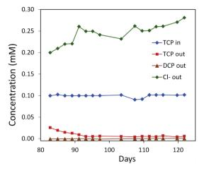
Fig. 6 Degradation of TCP by a mixed culture of *P. putida* strains MC4-5221, MC4-5221, MC4-1331 and *A. radiobacter* AD1 in a laboratory-scale aerated packed bed bioreactor operated in a continuous mode. Packing material was sintered glass and data were collected after an initial 80 day acclimation period. TCP loading rate 0.40-0.44 mg  $h^{-1}\,l^{-1}$ ; residence time 23 h; removal increasing to 95%.
