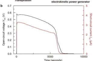
Fig. 1 TEPG. (a) Transpiration of plants (left) and the electrokinetic power generator whose operation resembles the transpiration of plants (right). (b) Measured  $V_{\rm OC}$  and  $I_{\rm SC}$  from the 120 k $\Omega$  TEPG generated by dropping 0.25 mL of DI water.
