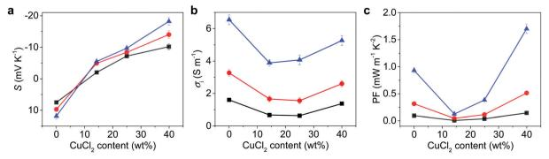
Fig. 2 Thermoelectric parameters of NPC films. (a) Seebeck coefficient, (b) ionic conductivity, and (c) power factor of NPC films at different RH values (%) and CuCl<sub>2</sub> contents. Black: 60% RH, red: 70% RH, blue: 80% RH. Error bars indicate the s.d. of three experimental replicates.
