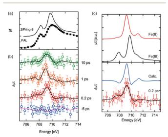
Fig. 2 Fe L<sub>3</sub> edge XAS spectrum of the hematite thin film (a), the transient Fe L<sub>3</sub> edge XAS spectra of photoexcited hematite at several delay times (b) and the calculated spectra of Fe L<sub>3</sub> edge XAS by the multiplet theory. The solid black line in panel (c) is the smoothed representation of the experimental data points that helps to clarify the spectral shape of the transient
