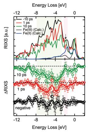
Fig. 4 2p3d RIXS spectra for -10 ps, 1 ps, 10 ps (top) and the difference RIXS spectrum for each delay time (bottom). The incident X-ray energy was 710 eV. The calculated spectra were normalised so that their elastic scattering intensities were half of the experimental spectra for clarity.
