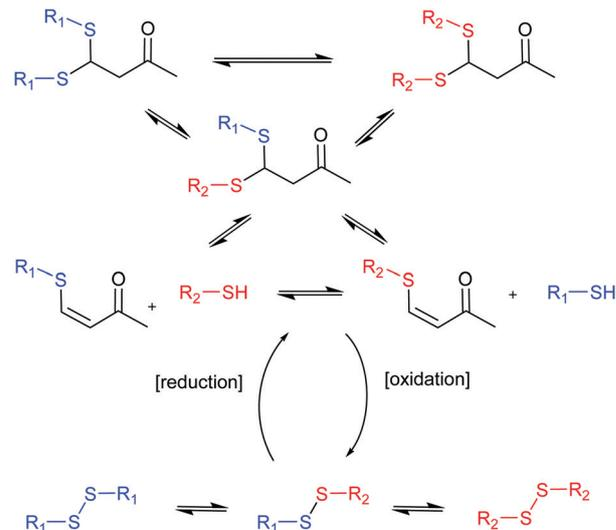
**Fig. 4** Antiparallel chemistries described by Otto.<sup>40</sup> The final state of the system between thio-Michael chemistry (top) or disulphide chemistry (bottom) can be switched by addition of reducing or oxidising agents.
