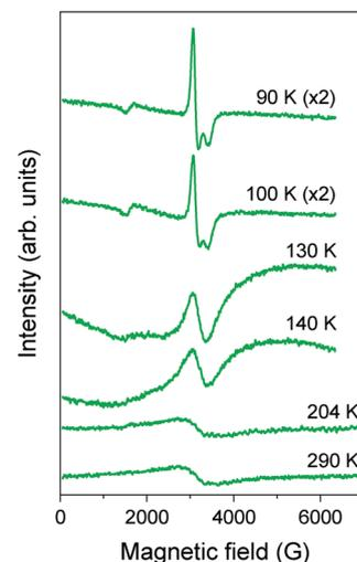
Fig. 7 Temperature dependence of ESR spectra of polycrystalline  $\text{Pt}_2(\text{EtCS}_2)_4\text{I}$ .<sup>35</sup>
