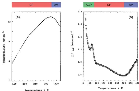
Fig. 5 Temperature dependence of (a) conductivity and (b) magnetic susceptibility ( $\chi$ ) of  $\text{Pt}_2(\text{MeCS}_2)_4\text{I}$  (AV: averaged-valence state, CP: charge-polarization state, ACP: alternate charge-polarization state). Adapted with permission from ref. 18. Copyright 1999 American Chemical Society.
