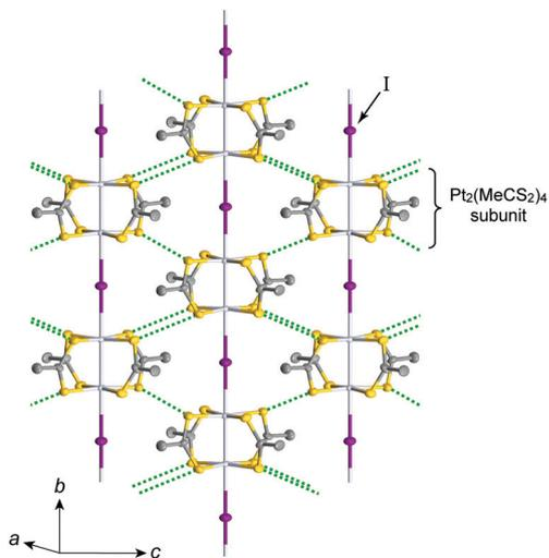
Fig. 4 Crystal structure of  $\text{Pt}_2(\text{MeCS}_2)_4\text{I}$  at room temperature,<sup>18,19</sup> where green dotted lines show heteroatomic S...S contacts between adjacent chains. Hydrogen atoms are omitted for clarity.
