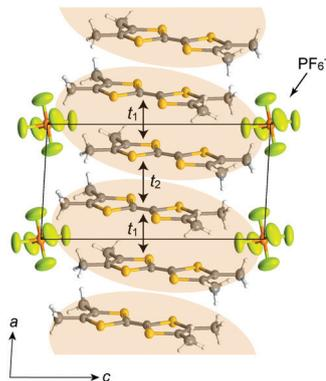
Fig. 14 Crystal structure of  $(\text{TMTTF})_2\text{PF}_6$  at room temperature viewed along the  $b$  axis, where the TMTTF dimers are indicated by orange ellipses.  $t_1$  and  $t_2$  are intra- and inter-dimer transfer energies, respectively.
