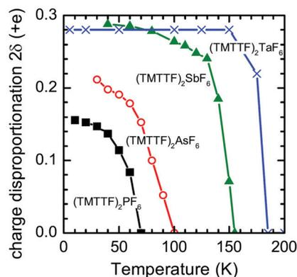
Fig. 18 Temperature dependence of the degree of charge disproportionation ( $2\delta$ ) of (TMTTF)<sub>2</sub>X with X = PF<sub>6</sub><sup>-</sup> (black closed squares), AsF<sub>6</sub><sup>-</sup> (red open circles), SbF<sub>6</sub><sup>-</sup> (green closed triangles), and TaF<sub>6</sub><sup>-</sup> (blue crosses), estimated from the IR spectra.<sup>85</sup>
