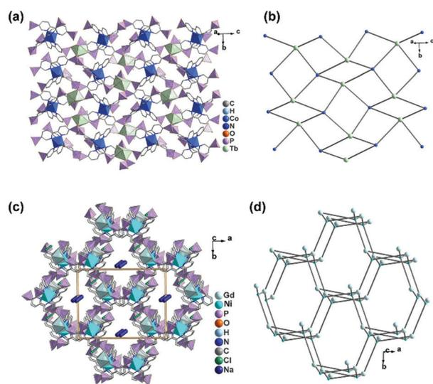
Fig. 15 (a) One layer and (b) layer topology of structure **67**. (c) Packing diagram and framework topology of structure **68**. The topologies in (b) and (d) are presented by the connections between the metalloligand centers and the lanthanide atoms. Adapted from ref. 67.
