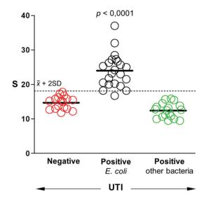
Fig. 5 Biosensor response when queried with a panel of patient samples that were E. coli positive ( $\geq 10^5$  cells per mL, black), E. coli negative, or positive due to an infection by another pathogen (green). Horizontal bars represent the mean. P-value was obtained with a Kruskall-Wallis test.
