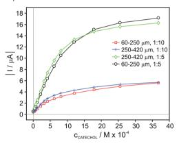
Fig. 1 Influence of (a) the applied potential and (b) paste composition and particle size on the recorded current.
