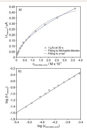
Fig. 6 (a) Plot of the absolute current change for increasing concentration of ascorbic acid in the presence of  $4 \times 10^{-5}$  M catechol concentration. (b) Calibration graph after data linearization.
