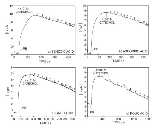
Fig. 4 Dynamic response of the sensors at a fixed concentration of catechol ( $4 \times 10^{-4}$  M) and gradually increasing the inhibitor concentration in the solution: (a) benzoic acid, (b) ascorbic acid, (c) gallic acid, and (d) kojic acid.
