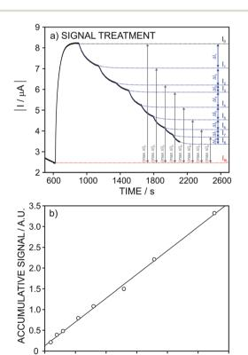
Fig. 8 (a) Recorded current response for increasing kojic acid concentration (black) and the corresponding extrapolated fitted curves (dashed blue line). (b) Calibration graph observed after linearization.
