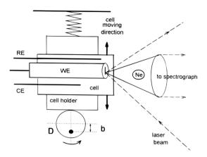
**Fig. 11** Schematic of a moving electrode cell. Ne is the Neon lamp and D is the rotating disk rotating around the axis represented by the black dot. Reprinted from the original work by Niaura *et al.*, <sup>140</sup> Copyright 1997, with permission from John Wiley and Sons.
