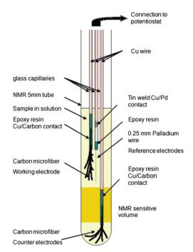
Fig. 15 Schematic of a three-electrode NMR-SEC cell with carbon microfibre WE and CE placed above and below the NMR detection area. Reprinted by permission from Springer Nature: from the original work by Bussy et al., 261 Copyright 2012.
