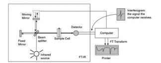
**Fig. 1** Schematic diagram by Pavia *et al.*<sup>10</sup> of an FTIR instrument. From Pavia/Lampman/Kriz/Vyvyan. Introduction to Spectroscopy, 4E. © 2009 Brooks/Cole, a part of Cengage, Inc. Reproduced by permission. http://www.cengage.com/permissions.
