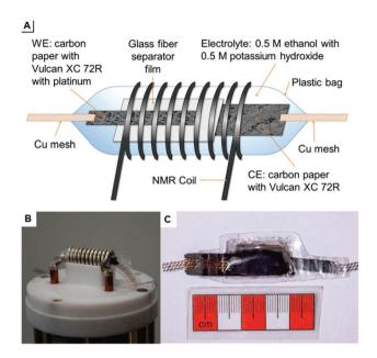
**Fig. 19** (A) schematic of a plastic pouch NMR-SEC cell and (B and C) photographs thereof. Reprinted from the original work by Richter *et al.*, <sup>276</sup> Copyright 2019, with permission from Creative Commons. Licensed under CC BY 3.0.
