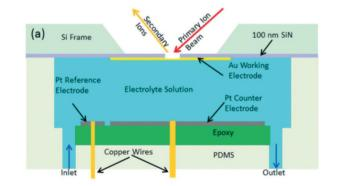
Fig. 26 Schematic of an EC-SIMS cell. Reprinted from the original work by Liu et al., 311 Copyright 2014 – Published by The Royal Society of Chemistry.
