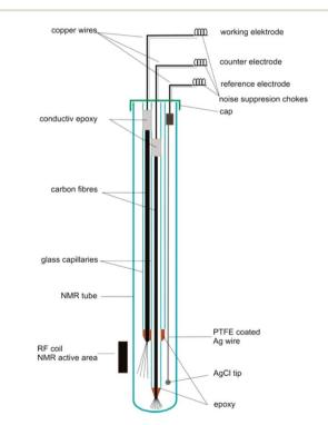
Fig. 14 Schematic of a three-electrode NMR-SEC cell with carbon fibre WE and CE, partially placed in the NMR detection area. Reprinted with permission from Klod et al.<sup>253</sup> Copyright 2009 American Chemical
