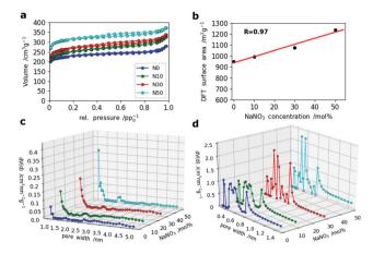
Fig. 5 (a)  $N_2$  sorption isotherms of all four samples, (b) correlation of DFT-derived surface area and  $NaNO_3$  content, (c) PSDs calculated by DFT (QSDFT (slit pore/cylindrical pore) model) based on the adsorption isotherms of  $N_2$  and (d) PSDs from  $CO_2$  adsorption measurements (NLDFT, Non-Localized DFT method).
