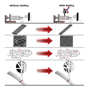
Scheme 1 Summary of effects of NaNO<sub>3</sub> in the electrospinning solution determined by various characterization techniques.
