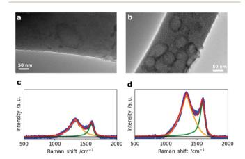
Fig. 3 TEM micrographs of (a) N0 and (b) N50 and corresponding Raman spectra of (c) NO and (d) N50.
