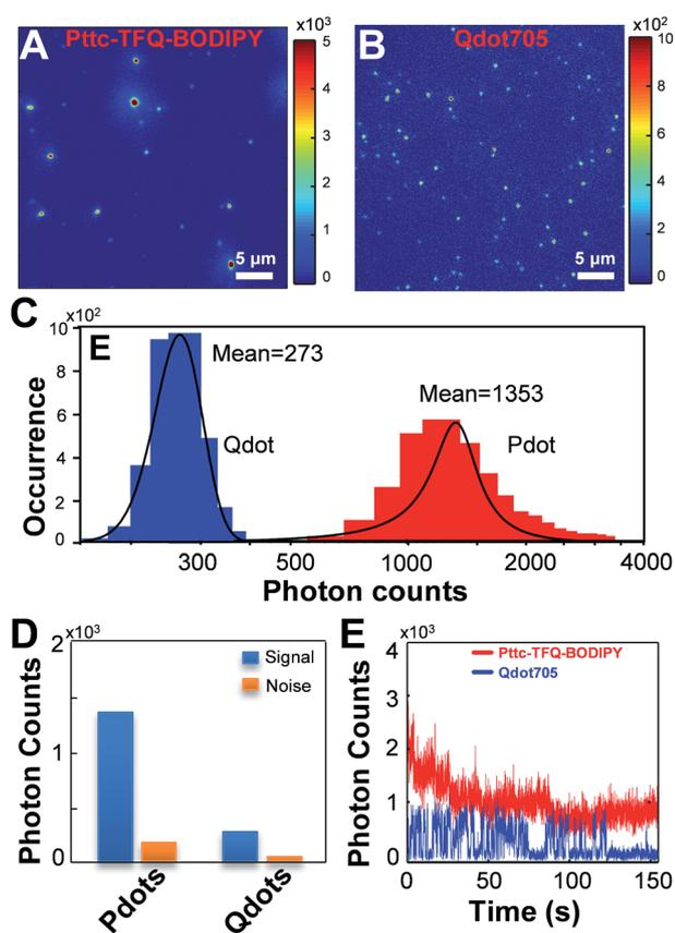
Fig. 7 Single-particle fluorescence images of (A) Pttc-TFQ-BODIPY Pdots and (B) commercial Qdot 705 quantum dots. Their corresponding (C) intensity distributions and (D) intensity histograms of signal to noise. (E) Single-particle photobleaching trajectories of Pttc-TFQ-BODIPY (red line) and Qdot 705 (blue line) under a 473 nm laser (1 mW). All of the images were acquired with a 473 nm laser under the same experimental conditions.
